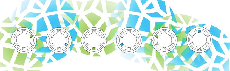
The stainless steel graphics panel at the base of the Aurorean is designed to project a series of patterns on the ground and surrounding objects. The position of the projections is directly related to the location of the light source inside the Aurorean. As the origin of the light source changes so will the position of the projection. This simulated movement helps to create a dynamic and interesting environment which is distinctly separate from its surroundings.
