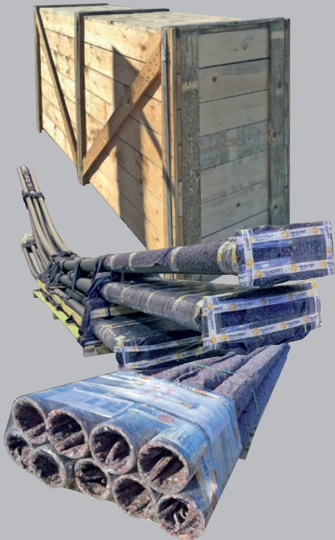
Packaging options for the transport and storage of different types of poles.
